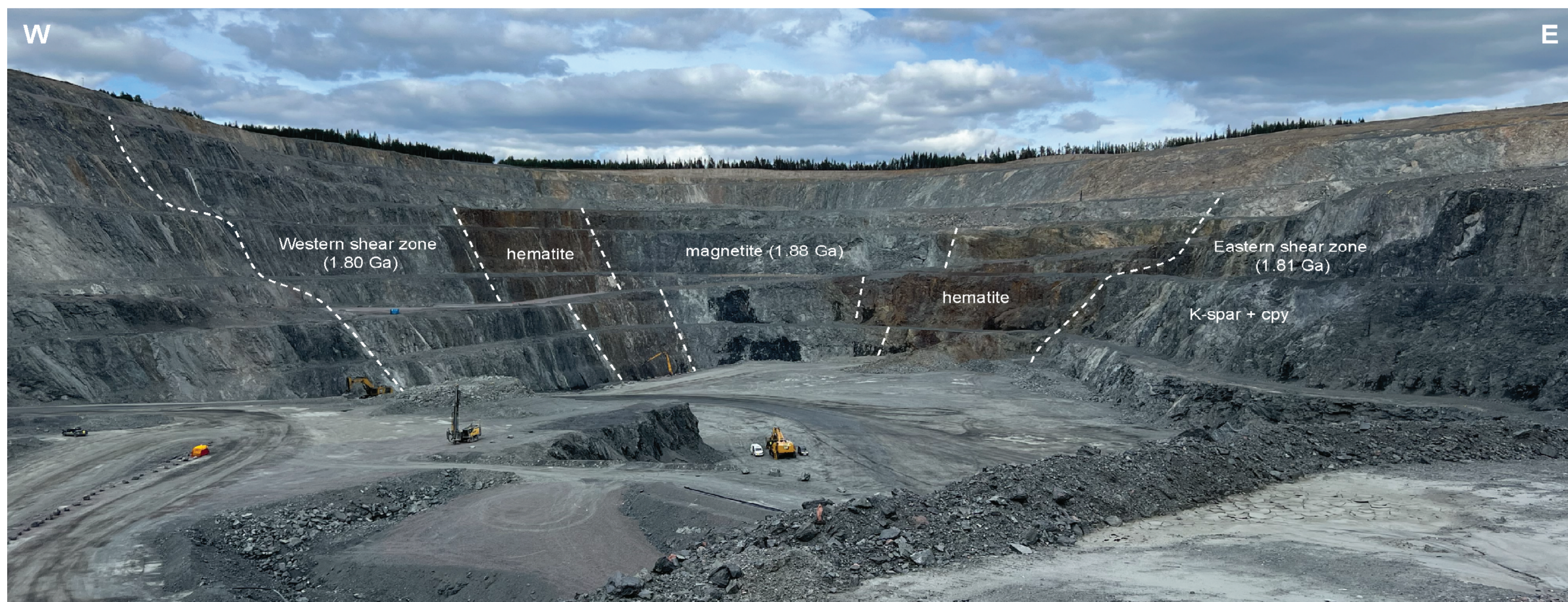
Fig. 3. Magnetite-(apatite) system crosscut by ca. 80 My younger shear-zone related IOCG mineralization. Levaniemi open pit, Kiruna.
